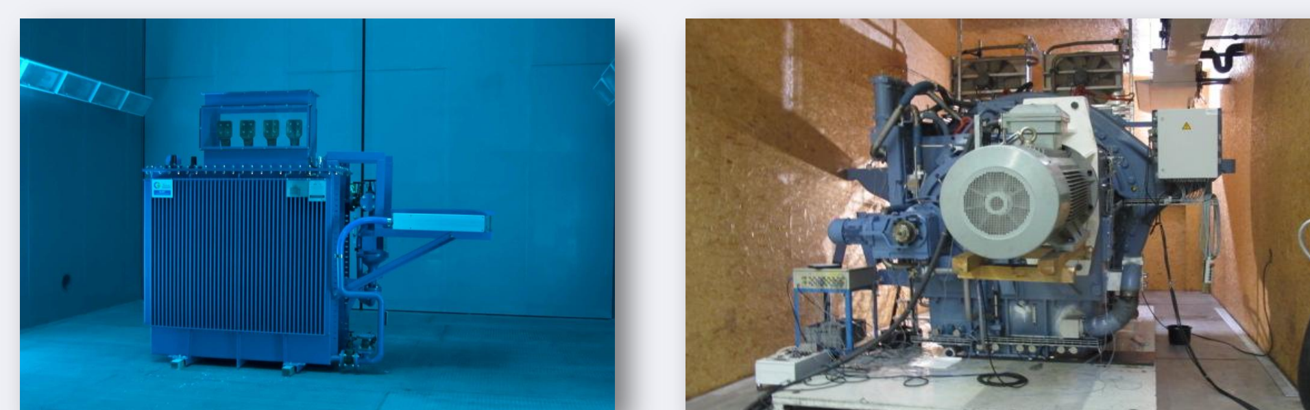
CG Power transformer in climate chamber & Cold start test ZF Wind Power Antwerpen NV
