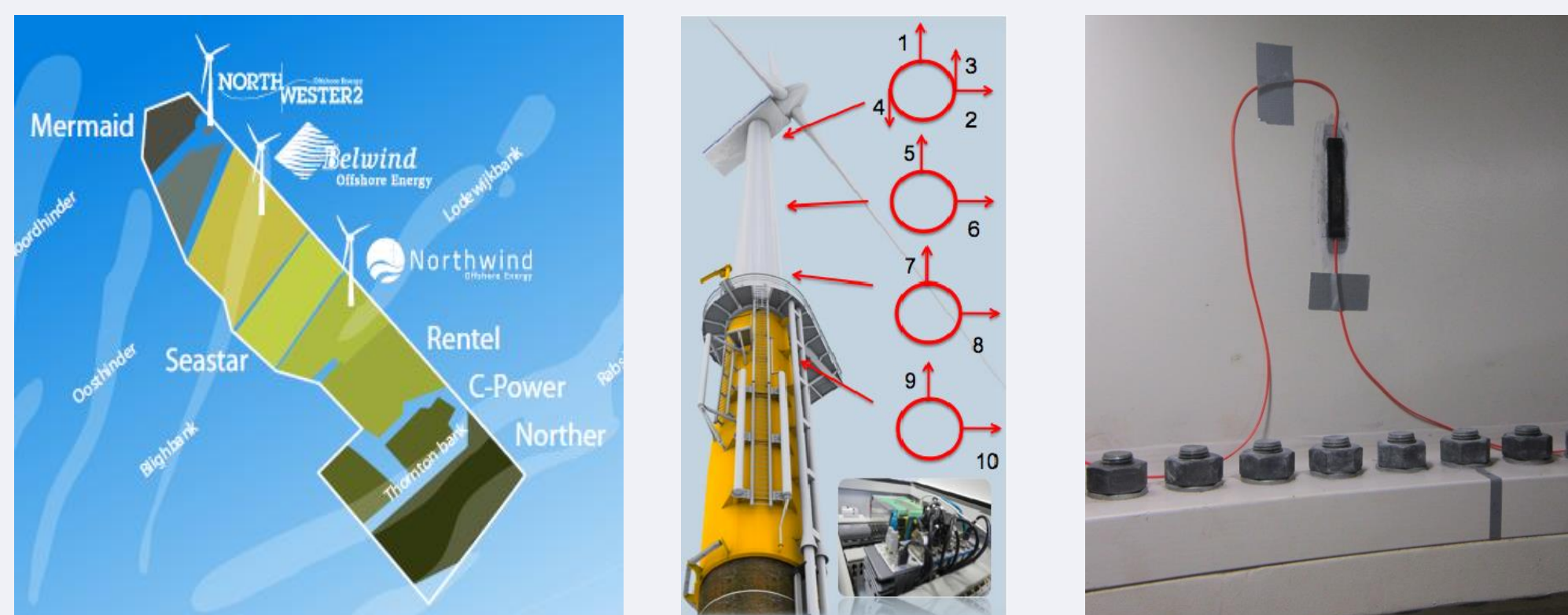
Figure 3: location Belwind wind farm (left), measurement locations of the acceleration measurements (middle), fiber Bragg grating sensors for strain measurements installed above the flange connection on 4 locations (right)
